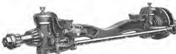
Heavy Type Timken Axle for Large Trucks.
